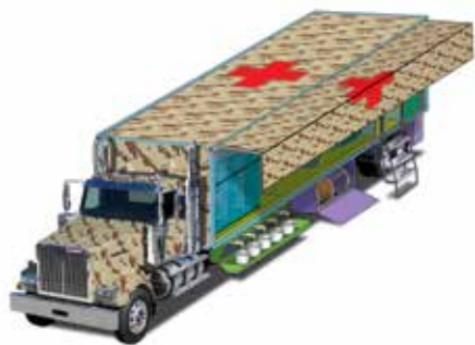
RETRACTABLE SIDE WALLS FUNCTION AS A PROTECTIVE AWNING
